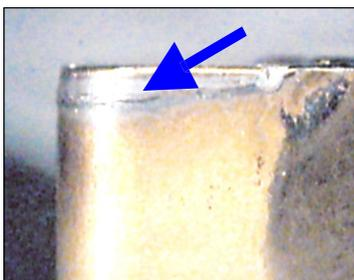
Flank wear is the preferred type of insert wear, symbolizing a normal insert wear over time. Rapid flank wear however can cause poor surface finish quality or an inconsistency in tolerances.
