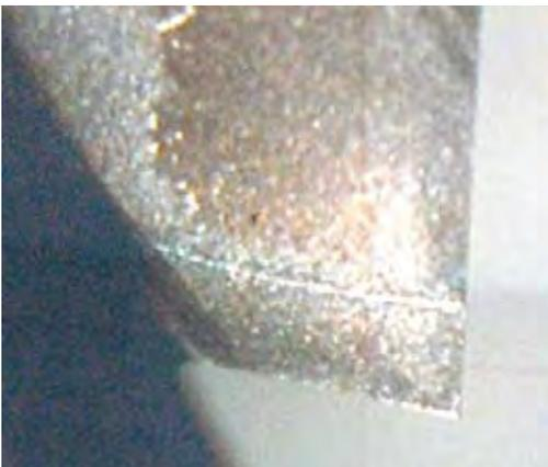
Thermal cracking, as its name suggests, is caused by extreme temperature fluctuations during milling. Adding a proper coating to an end mill is beneficial in providing heat resistance and reduced abrasion on a tool. HEM toolpaths provide excellent protection against thermal cracking, as these toolpaths spread the heat across the cutting edge of the tool, reducing the overall temperature and preventing serious fluctuations in heat.
