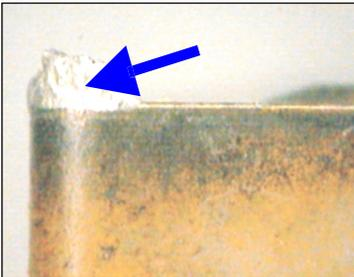
Built-up edge on an insert will cause poor surface finish and chipping cutting edge when the BUE is torn away.
