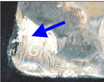
Excessive crater wear causes a weakened cutting edge and poor surface finish quality.
