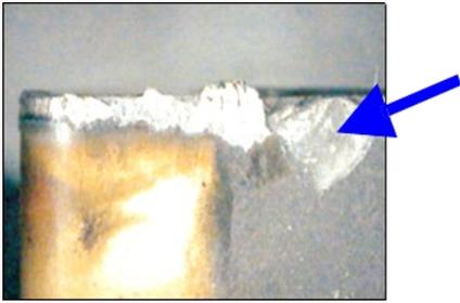
Notch wear typically causes poor surface finish and the risk of insert edge breakage.
