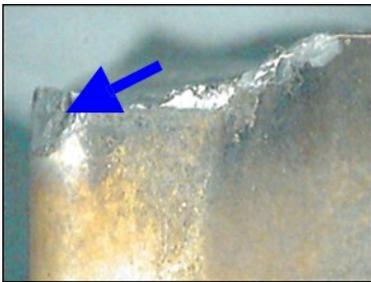
Cutting edge fracture not only damages the insert, but also can destroy the cutter body and/or the work piece itself.
