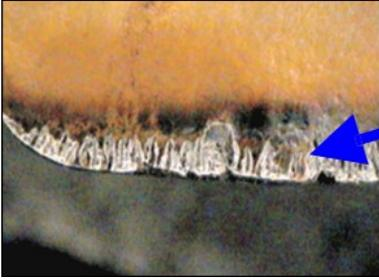
Thermal cracking shows up as small cracks perpendicular to the cutting edge, resulting in chipping and poor surface finish.
