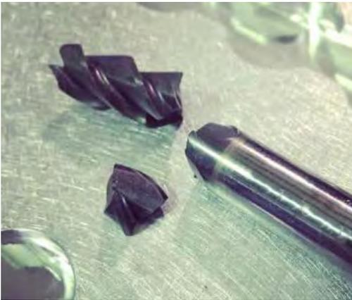
Adjusting the speeds, feeds, and depth of cut and checking the setup for rigidity will help to reduce fracturing. Optimizing coolant usage can also be helpful to avoid hot spots in materials which can dull a cutting edge and cause a fracture. HEM toolpaths prevent fracture by offering a more consistent load on a tool. Shock loading is reduced, causing less stress on a tool, which lessens the likelihood of breakage and increases tool life.
