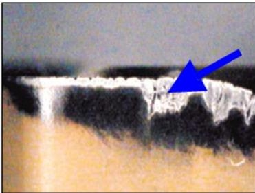
Characterized by small chips on cutting edge, leading to poor surface finish and excessive flank wear.
