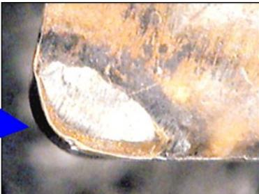
Plastic deformation of the cutting edge is characterized by a depression of the edge, or an impression on the insert flank, leading to a poor chip control, poor surface finish and insert breakage.
